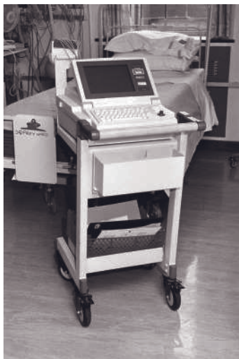
Figure 10.1 Electrocardiograph or ECG machine.
