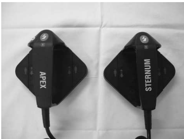
Figure 12.3 Handheld paddle electrodes.
