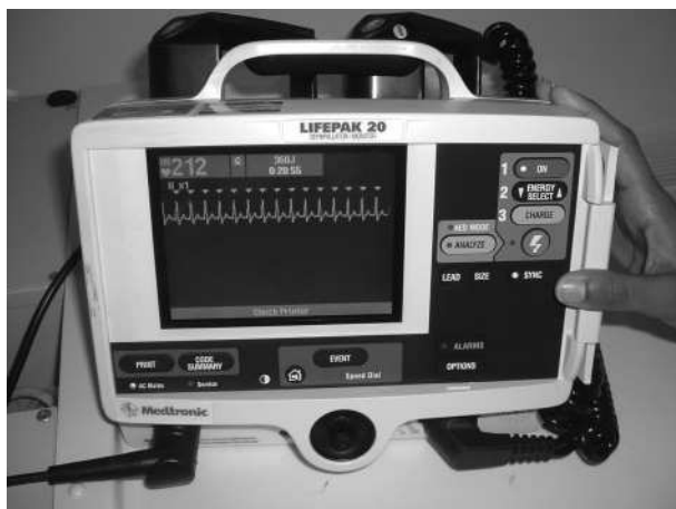
Figure 12.6 Electrical cardioversion: activating the synchronised button.
