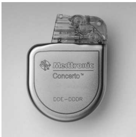
Figure 12.9 Implantable cardioverter defibrillator (ICD).
