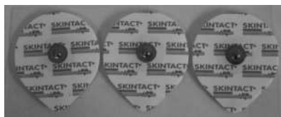
Figure 2.10 ECG electrode. Reproduced by kind permission of Ambu.
