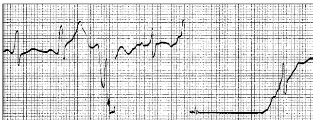
Figure 2.18 Loose electrode. Reproduced by kind permission of Ambu.
